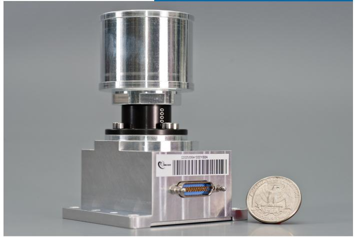
Auriga is the very last innovative Sodern star tracker specifically made to meet cost reduction, increased production rate and technical performance objectives of the satellites constellations emerging market.
