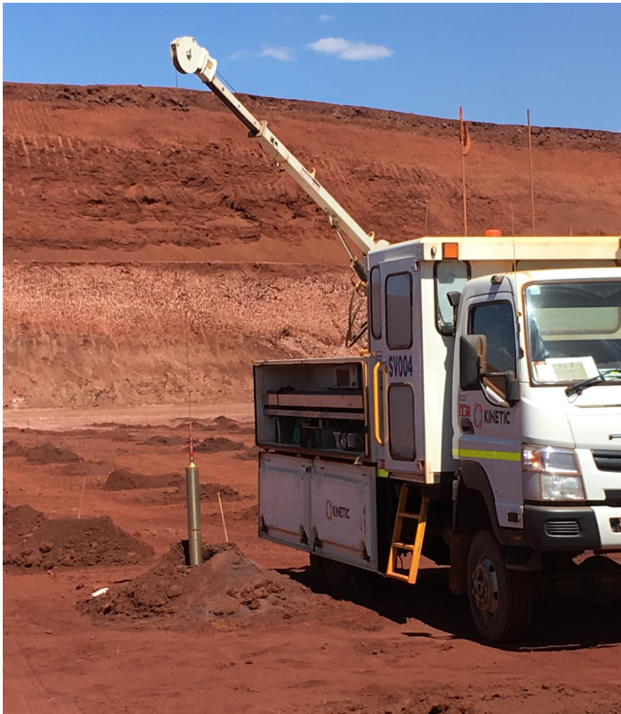
Open-pit blast hole logging with FastGrade™
